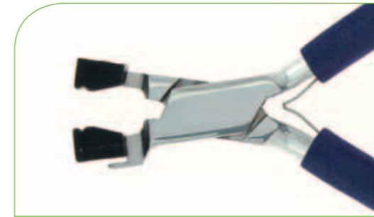
Plier to crimp plastic riders Ref: PIN018 «Silhouette» Type - 2 fixed nylon jaws Stainless steel - △ 130 gr - ▷ 145 mm Replacement jaws - Ref: PINP18
