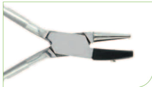
Inclination conical plier Ref: PIN004 To adjust pad arms, temples and joints Conical mandal jaw and nylon jaw of 7 mm. Stainless steel - △ 100 gr - ► 140 mm Replacement jaws Ref: PINPD4
