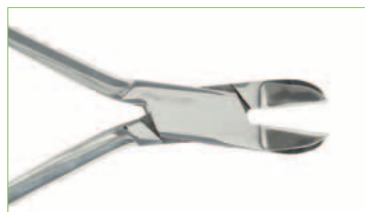
Side cutting semi short Ref: PIN011 Nickered steel - end semi-flush cutting Cutting capacity: half hard mandal Ø1.5 mm △ 100 gr - ► 140 mm
