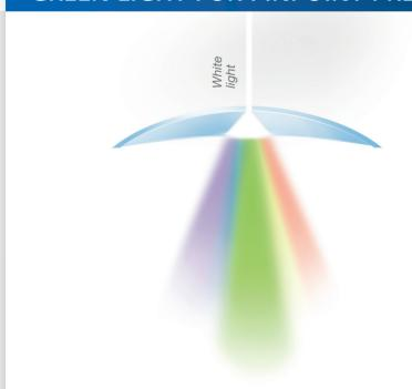
The ALM 500 and ALM 700 use a green light beam\* that reduces measurement drift due to light deviation by the lens.
